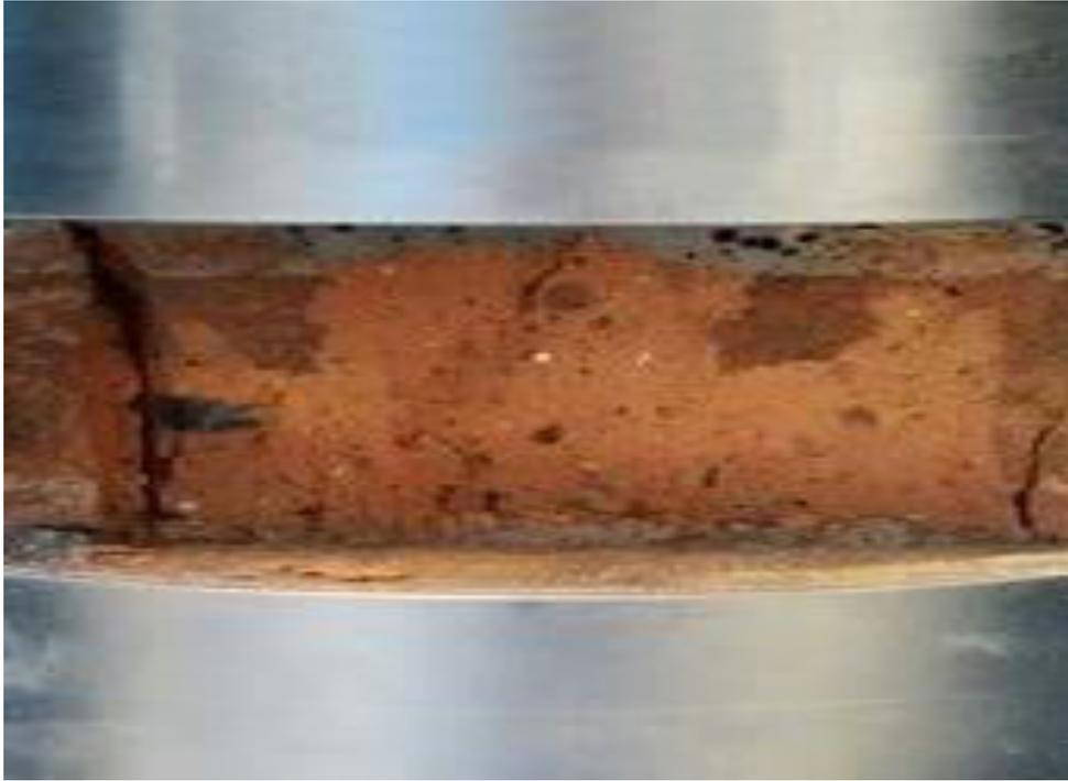
Fig.4.4 Testing Of brick Under CTM
