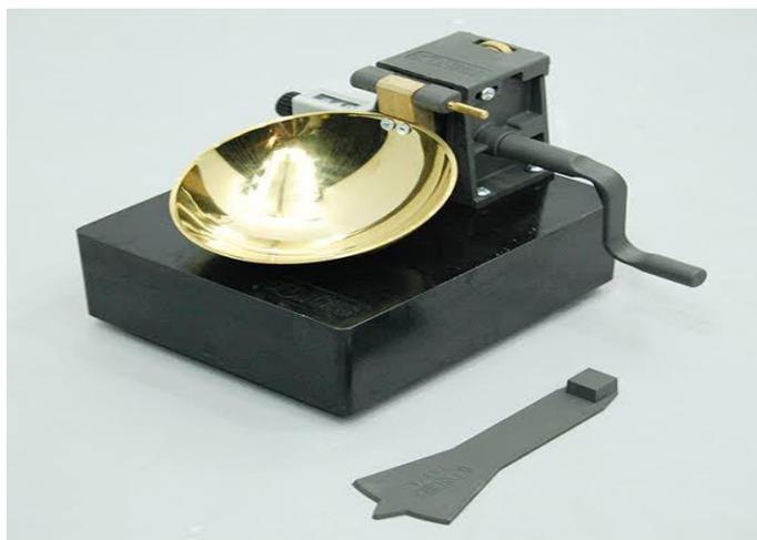
Fig.4.2 Liquid Limit Test
